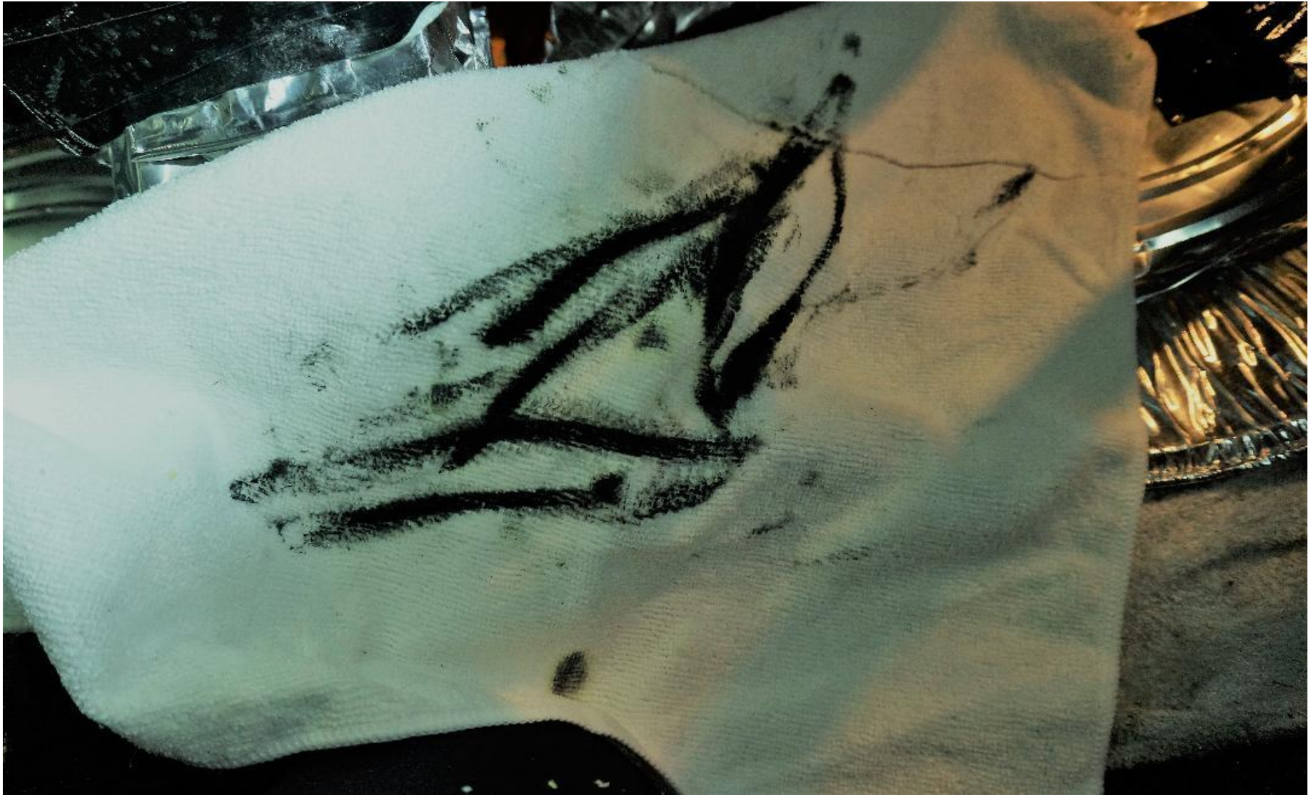
Chain wipe down after first 400km interval. The lube was not that colour when it went on.
