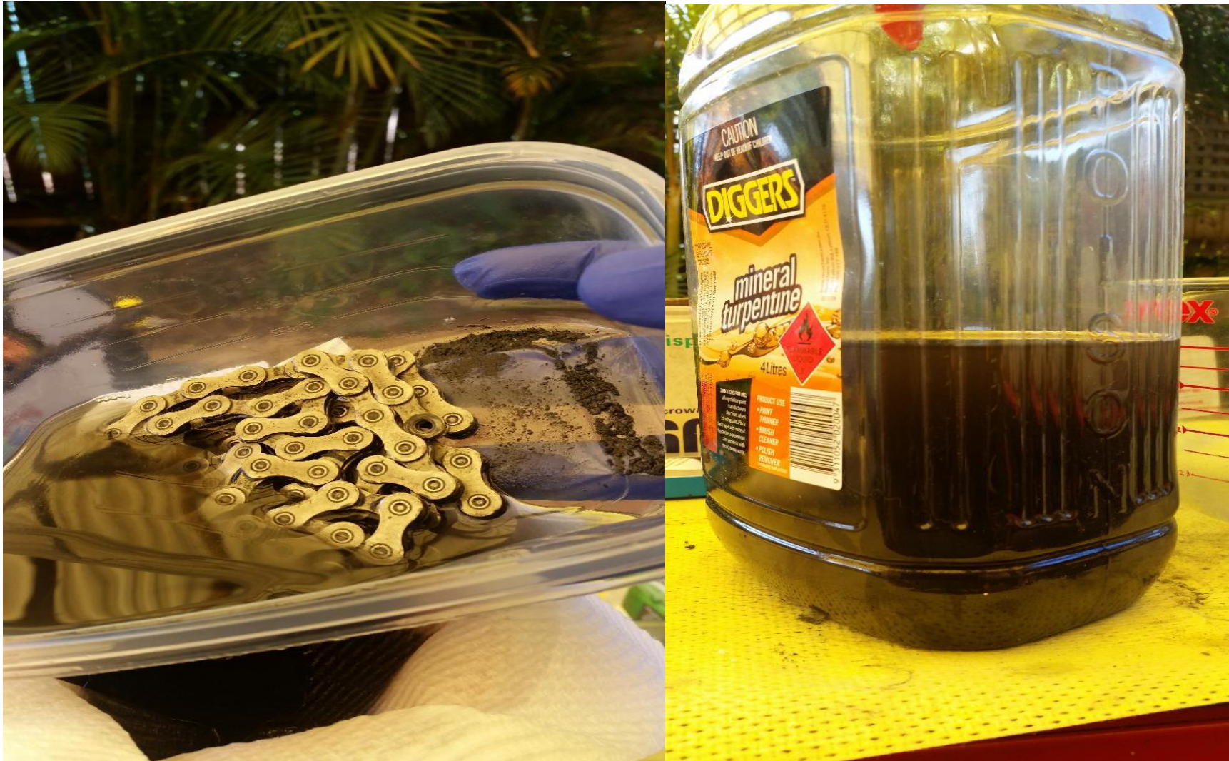
End of main test cleaning after 3,800km. A lot of grit flushed out, and nearly 2 litres of mineral turps before turps coming out fairly clear from agitated rinse.
