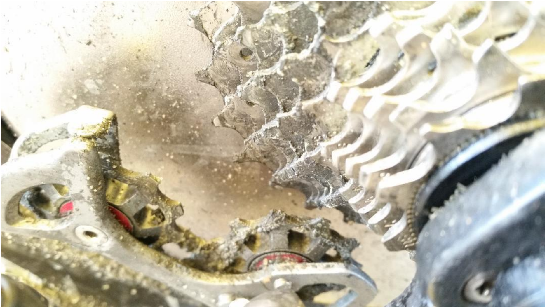
End of test – Jockey wheels still accumulated some gunk in 3,800km.
