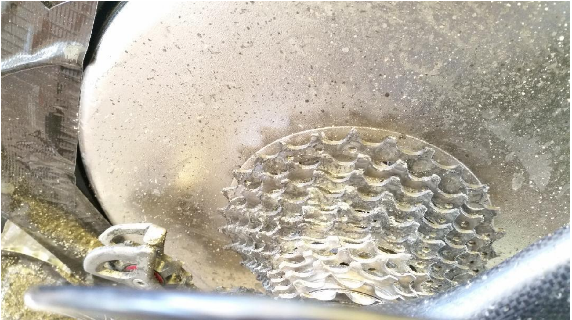
End of test – the 6 cogs in use during test
